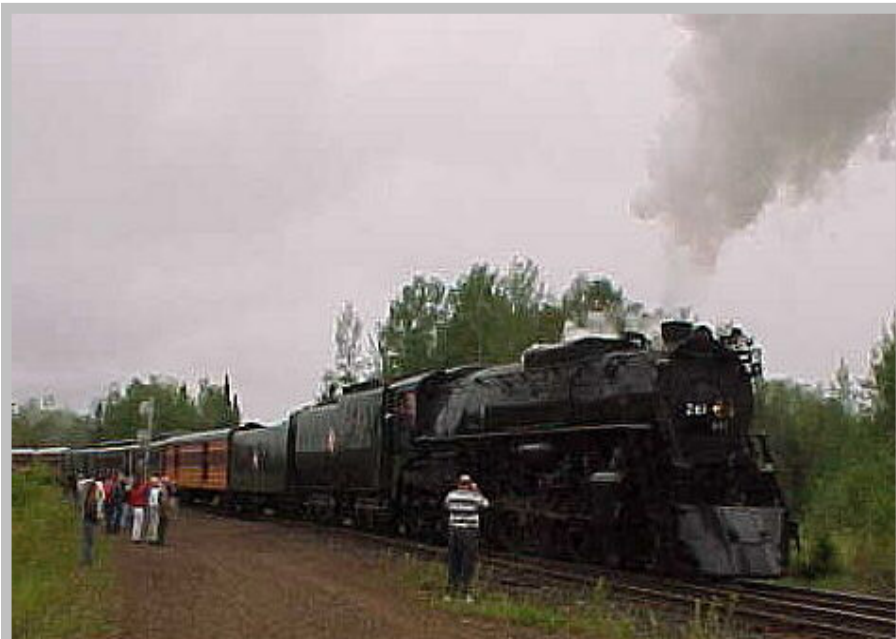
Milwaukee RR 4-8-4 #261 near Iron Junction on s special DM&IR circle trip out of Duluth, MN. 216 had 21 cars and nearly 1000 passengers on it's drawbar. September 2, 2000
